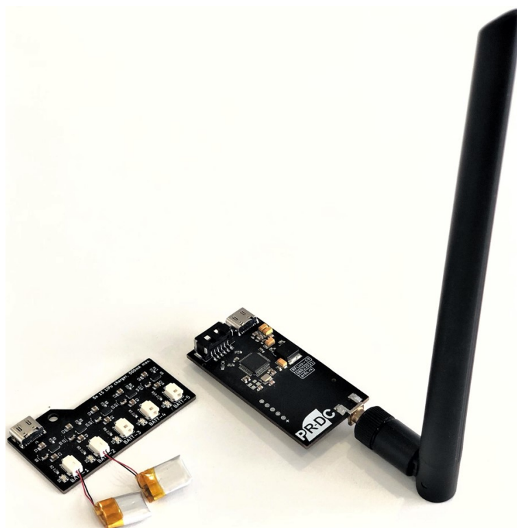
Figure 5 - Fast battery charger and receiver
